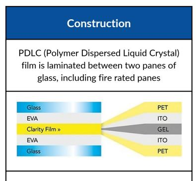
Clarity Film (PDLC) consists of a GEL Center Layer between two ITO Layers and two PET Protective Layers.
