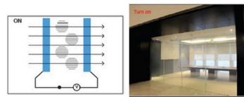
When electricity is applied, the liquid crystal molecules line up, the incident light passes through, and Clarity looks clear.
