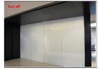
When the power is off, the liquid crystal molecules are randomly oriented which scatters incident light, and Clarity becomes translucent.
